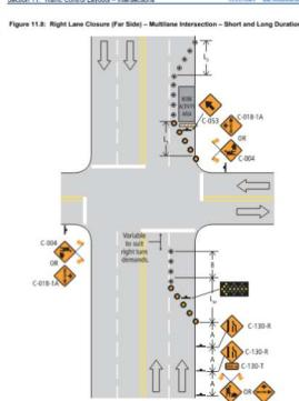
Figure 11.8: Right Lane Closure (Far Side) - Multilane Intersection - Short and Long Duration
